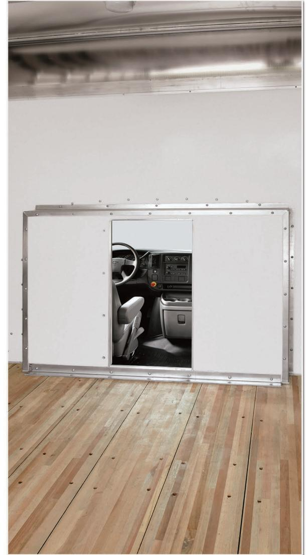
An option for a recessed bulkhead that provides more room in the cab and easier positioning of the seat.
