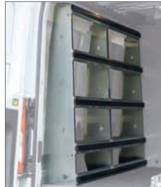
Transport glass on upper portion of rack when the bottom ledge is occupied. Row of E-track required (Sold Separately).
