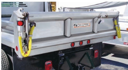
Vertical tailgate allows easy attachment of spreaders during winter.
