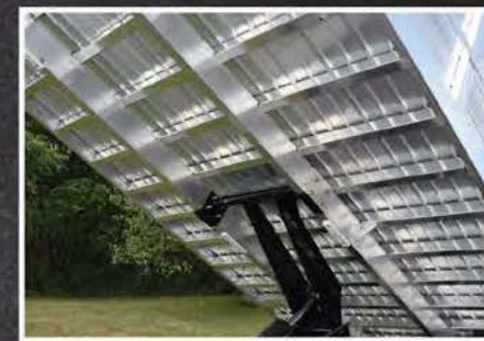
Standard HD Subframe with 12" OC Cross Members
