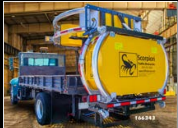
Custom flatbed with Scorpion Atenuator
