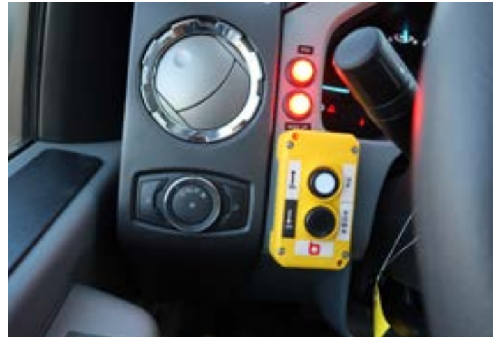
Dash-mounted LED "Body Up" Safety Light and Push Button Hoist Up-Down Controller
