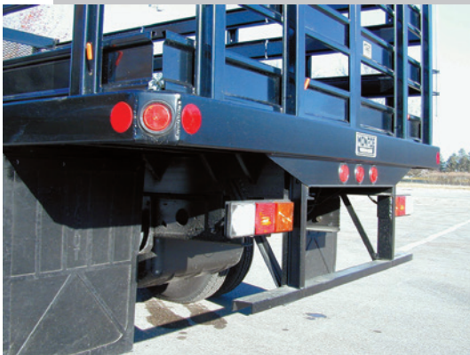
Rubber mounted lights to FMVSS specifications
