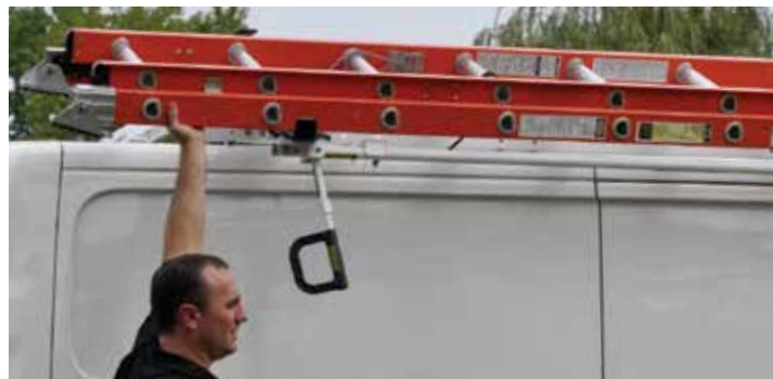
Lift ladder off the rear bracket.
