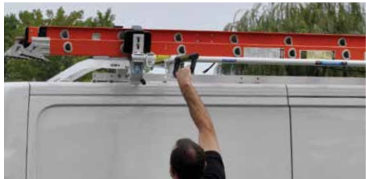
Pull to release the handle, swing out and down to lower ladder.
