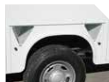
WHEEL CHOCK HOLDER - FENDER SKIRT
