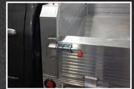
Drop Down Sides with Spring-loaded Latches
