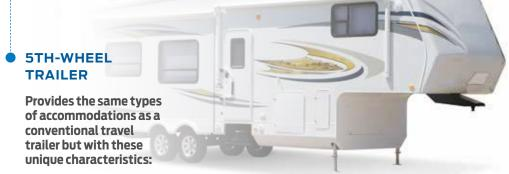
The forward raised portion is designed to extend over the box of a pickup truck
