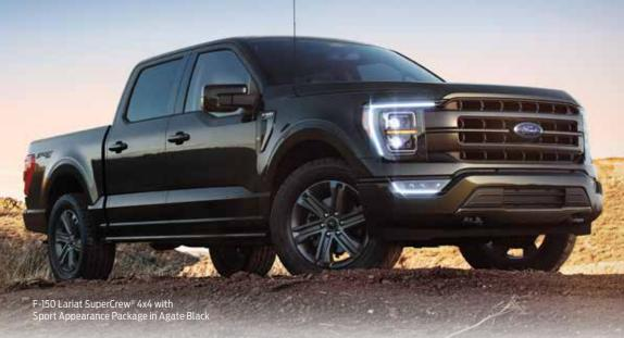
The all-new 2021 F-150 Pickup is a true workhorse and is purpose-built to handle the toughest jobs. A fully boxed high-strength steel frame with a high-strength, military-grade, aluminum alloy body to save weight and add capability, helping F-150 tow best-in-class maximum available 14,000 lbs.1 and deliver a best-in-class available payload rating of 3,325 lbs.<sup>2</sup>
