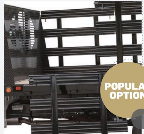
Accommodate oversized loads and allow **accessibility** from any direction with removable stake sides.
