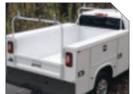
OVERHEAD LADDER RACK
